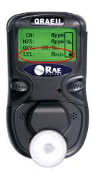
At a concentration higher than 10-20% LEL an acoustic and optical alarm is given. When 100% of the lower explosion limit is measured, this means that the mixture can be ignited. For such an ignition only a source of sufficient energy is needed.
