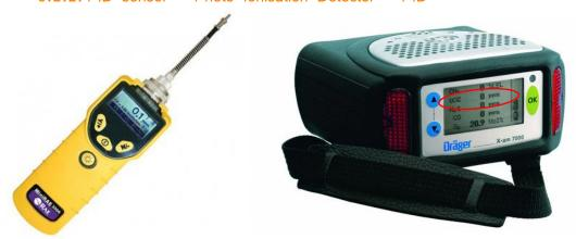
A PID meter continuously detects the concentration of volatile organic compounds (VOCs) present, toxic gases and/or vapors expressed in parts per million (PPM). However, a PID meter does not detect gas specifically, all VOCs in the gas sample to be measured are displayed as one common values on the display of the PID detector.
